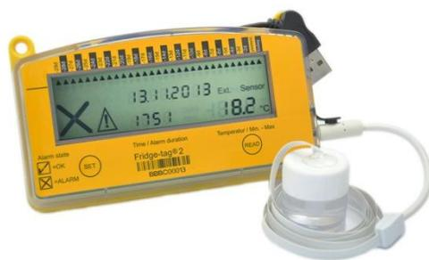
*Fig. 4 – The Fridge-tag 2 temperature monitor. The device records temperature for 30 days from a digital thermometer placed in a dummy vaccine vial. The USB shown behind allows clinicians to upload data to a computer to check for any temperatures breaches that may have been missed. Image from Thermco Products.*
