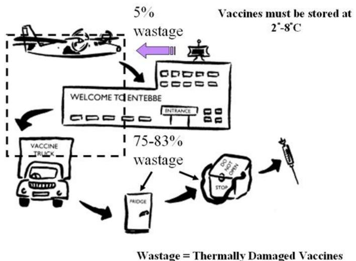
Fig. 1 - Diagram of the current ‘cold chain’ vaccine transport system. Percent wastage indicates what percent of vaccine spoiling happens in the corresponding stage. Note that the highest amount of wastage happens in the storage and mobile refrigerator stages of transport, and hence more efforts are focused on those areas. Image from One World Medical Devices.
