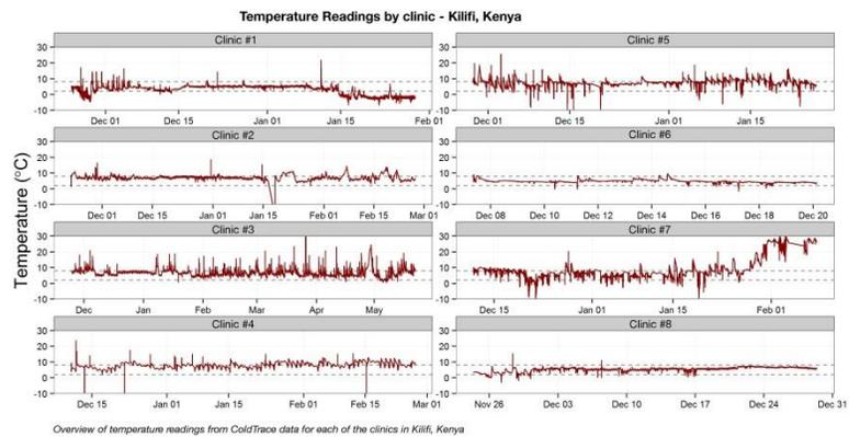
*Fig. 5 – Temperature recorded by a ColdTrace vaccine fridge monitor from eight clinics in Kilifi, Kenya. Many clinics show large deviations from the accepted cold chain range (shown by gray dashes) as well as cyclic spikes out of range, indicating severe weak points in refrigeration systems. Image from Datakind.*
