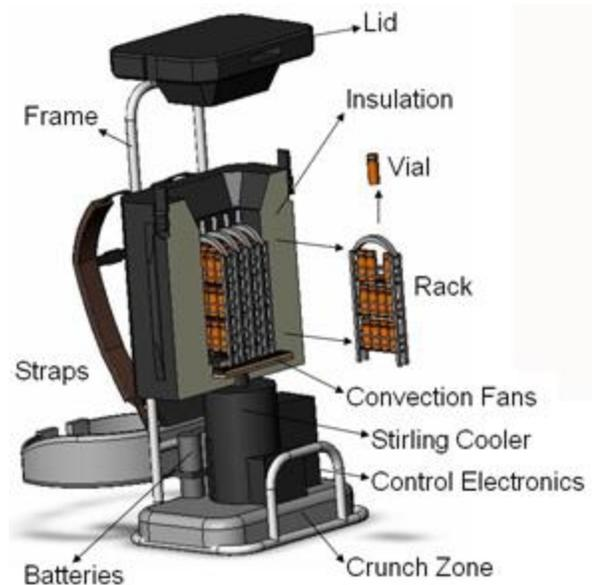
Fig. 3- The VacPac mobile vaccine refrigerator. Designed to be worn as a backpack, stores 1200 doses of vaccine, and rechargeable batteries allow for 18-24 hours of cooling per charge. Image from One World MD.
