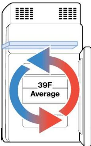
*Fig. 2- Diagram of the Sure Chill refrigeration system. The refrigerator uses an ice bank above and the principle that water is heaviest at 4°C (39°F) to keep a constant supply of water at that temperature flowing around the chamber. This approach can continue refrigeration at a stable temperature for up to 10 days without power. Image from Tozzi.<sup>25</sup>*
