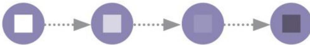
*Fig. 4 – The Vaccine Vial Monitor, a sticker developed by PATH to help clinicians determine if a vaccine is fit for use. The center square gets darker as the vaccine is exposed for longer times or to more intense temperatures outside the cold chain, and the vaccine is determined unfit for use when the color of the square matches the color of the circle. Image from PATH (36).*
